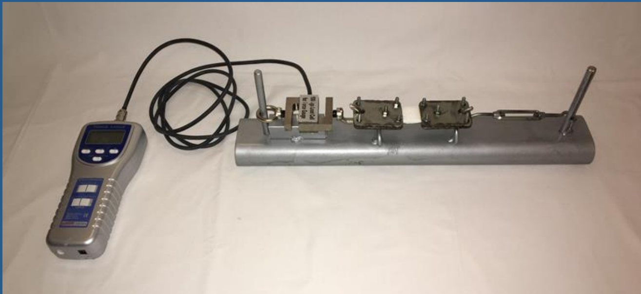
Figure 2: System of clamps and screws used for graduated distension of the skin
